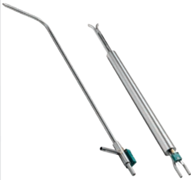
Gas flow velocity measurement (m/s) by means of pitot tubes
